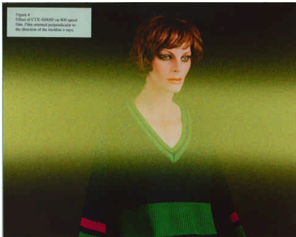
Figure 4 – Effect of CTX-500SP on ISO 800 speed film. Film oriented perpendicular to the direction of the incident X-rays
