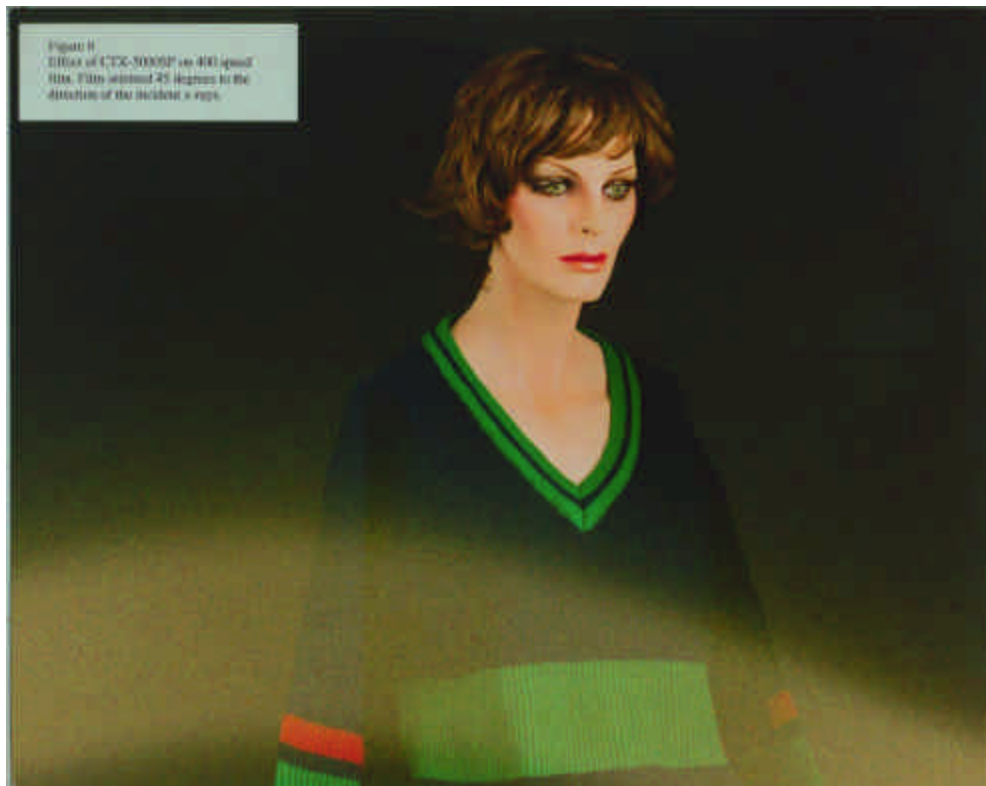
Figure 6 – Effect of CTX-500SP on ISO 400 speed film. Film oriented 45° to the direction of the incident X-rays
