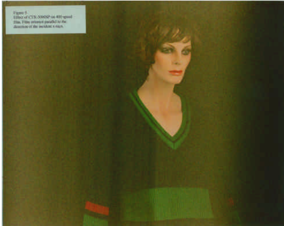
Figure 5 – Effect of CTX-500SP on ISO 400 speed film. Film oriented parallel to the direction of the incident X-rays
