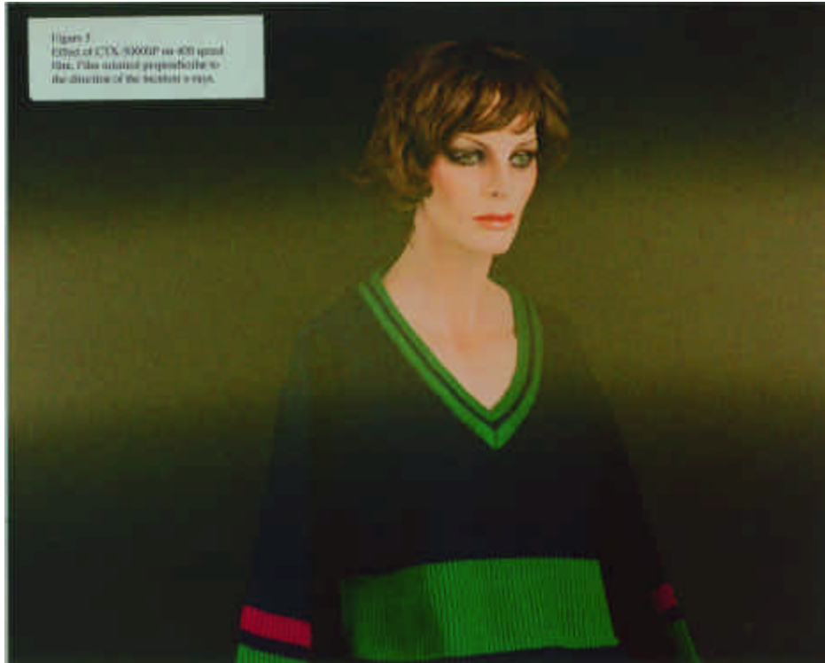
Figure 3 – Effect of CTX-500SP on ISO 400 speed film. Film oriented perpendicular to the direction of the incident X-rays
